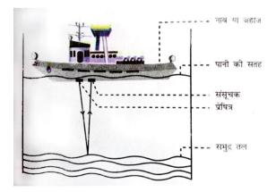
**Figure**: Ultrasound transmitted by the transmitter and received by the detector.
