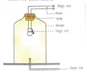
**Image:** Bell jar used to show that sound cannot propagate in vacuum.
