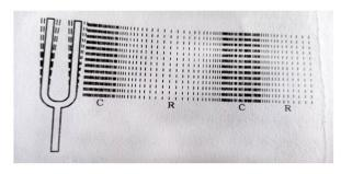
**Figure:** A vibrating object producing a series of compression (C) and rarefaction (R) in a medium.
