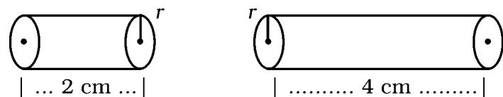
In the figure, resistivities of two conductors of same material are  $\rho_1 \Omega\text{-m}$  and  $\rho_2 \Omega\text{-m}$  respectively. Write the value of ratio of  $\rho_1$  and  $\rho_2$
